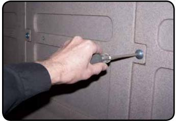
All the panel screws can now be tightened. TIP: Before tightening screws, walk around the camper/shelter and pull the strap in the direction of the buckle to make sure it is uniformly tight. Re-cinch the buckle.
