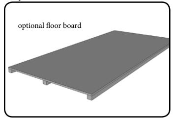
Prepare a floor board or trailer floor. 1/2" to 3/4" plywood or OSB is recommended. 2"x2" support runners can be used but are not necessary. Floor should be flat and stable.
