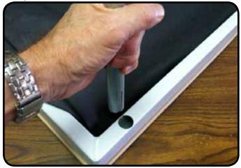
Insert the bench legs into the holes in the bottom of the bench frame. This is a tight fit and may require some force.
