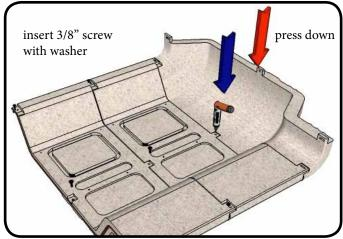
While pressing down on the edge of the corner panel to compress the seal, insert the 3/8" center screw and washer. Repeat on the other corner. (TIP: If lining up the hole is difficult, swap corners)
