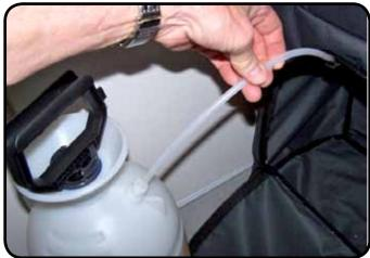
Insert the dip tube into the pressure bottle and screw the plastic nut down tight. To fill with water the dip tube can be removed and the bottle carried. Rotate the pump handle to open the bottle. Pump the handle to create water pressure.
