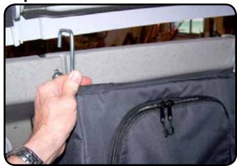
Unlatch the roof and raise it enough to hang the cabinet hooks over the top of the side panel. Hooks should line up with the joint in the panels.
