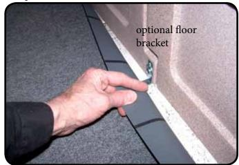
Optional "L" shaped floor brackets are used to attach the walls to a floor board if the floor is intended to stay with the camper when removed from the trailer.
