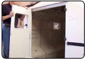
The door can now be hung by simply setting them on the hinges. They are just as easily removed. The left door has top and bottom sliding locks that anchor the door. These bolts must be in the locked position before closing the right door.
