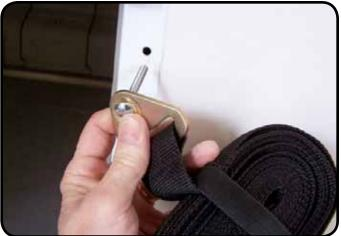
Attach the assembly/safety strap to the right side of the doorframe using the bolt and wing nut. The angled portion of the slotted strap fitting should be facing away from the door frame.
