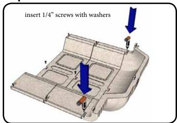
Lay the side panels flat and attach a corner panel with the top and bottom 1/4" screws and washers.
