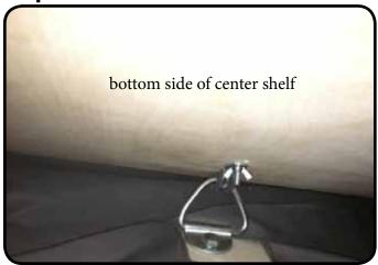
Place the middle shelf so the back of the shelf rests on the wall panel and the front channel fits over the shelf rod between the legs. Attach the C-clamp to the wall panel D-ring and tighten the screw while holding the wingnut.
