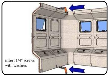
To add more panels, start by inserting the top and bottom 1/4" screws and washers.
