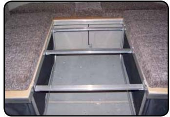
Three support bars are supplied for converting the dinette into a bed. Place the support bars between the benches using the end brackets to hang on the bench frame.
