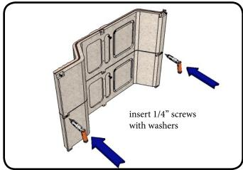
Stand a side panel on edge and stack another side panel on top. Insert the top and bottom panel 1/4" screws and washers (TIP: Swap panels if inserting screws is difficult.)
