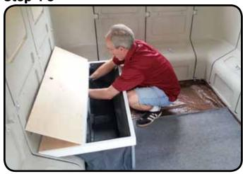
Line up the holes in the bench seat with the tiedown rings on the panel and thread the strap through the tiedown ring and insert it in the buckle provided on the bench. Pull the strap tight..
