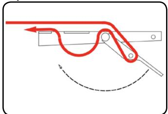
Use the above illustration to thread the strap into the buckle. If the strap is not threaded correctly it will not cinch up the belt or hold it firm.
