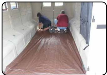
Roll out floor liner and attach it to the front panel screws through though the grommets provided in the liner.
