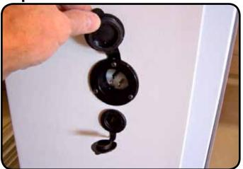
There are two receptacles on the outside of the door frame. Plug in an extension chord to the to one for 120 volt power. Plug in a battery, generator or solar panels for 12 volt power.
