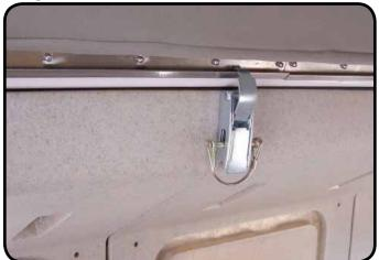
Insert the locking pin or screws with wingnuts into the roof clamps whenever travelling. This will prevent the clamp from vibrating open or the screw from backing out.
