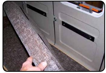
Using the short 1/4" screws, attach the Velcro bars to side panels to hold the seat back cushions in place.
