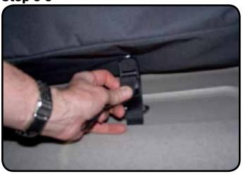
Attach the bottom strap to the tiedown ring on the side panel. Pull the strap tight for a snug fit.
