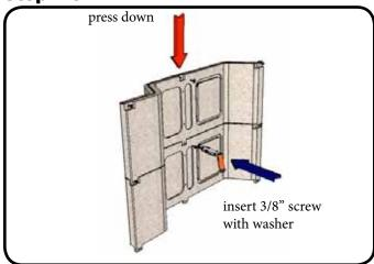
While pressing down on the center of the top panel, insert the 3/8" center screw and washer. (TIP: If you have a 4' wide unit you will be using the modified wide front panel instead of two standard side panels.)
