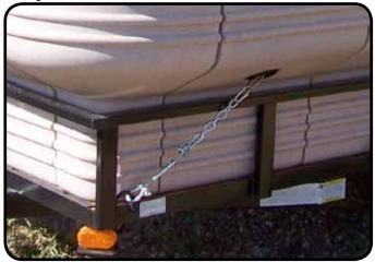
Use the external tiedown rings to anchor the camper/shelter. Tiedown straps or chains with turnbuckles may be used. Tiedowns should be snug with no slack. DO NOT over tighten.
