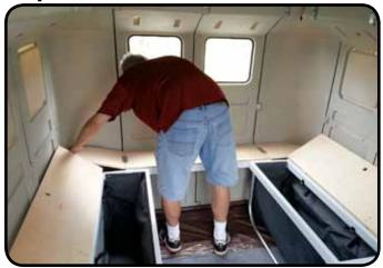
Open the bench seat lids and place the end shelf across the end wall panels. The back of the shelf rests on the panels while the front hangers fit over the bench frame.
