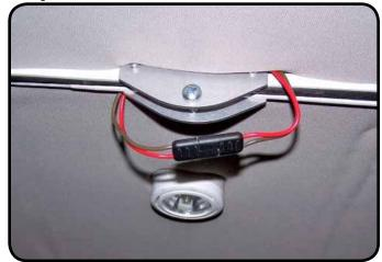
Connect the ceiling lights in each section with the joining plugs.
