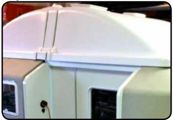
For side door campers or longer roofs, insert the center sections that came with the kit.
