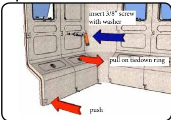
To compress the seal while inserting the center 3/8" screw and washer, pull on the tiedown ring of attached panel while holding the opposite corner of the new panel stationairy.
